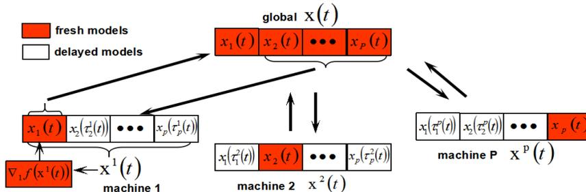
Figure 1: The algorithm msPG under model parallelism and stale synchronism. Machine  $i$  keeps a local model  $\mathbf{x}^i(t)$  that contains stale parameters of other machines (due to communication delay and network latency). These local models are used to compute the partial gradient  $\nabla_i f(\mathbf{x}^i)$  which is then used to update the parameters  $x_i(t)$  in each machine. See Section 5 for an economical implementation of msPG.
