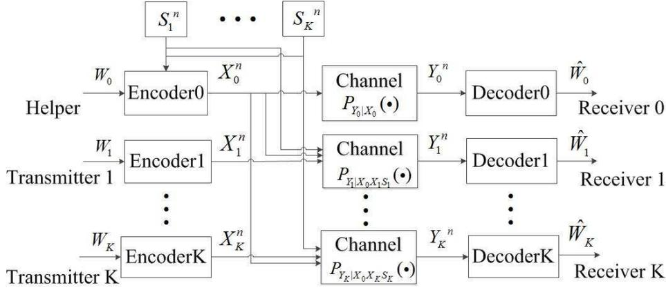
Fig. 2: Parallel Gaussian channel model with a common state-cognitive helper.
