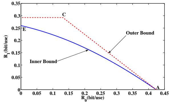
(b)  $P_1 < 1$  with  $P_0 = 0.8$  and  $P_1 = 0.5$ Fig. 5: Inner and outer bounds for case 2 with  $P_0 \geq P_1$ , which match partially on the boundaries
