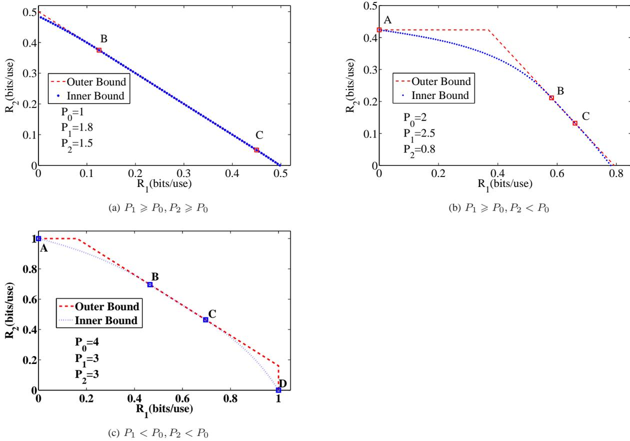
Fig. 8: Inner and outer bounds for the Gaussian channel of model III with  $K = 2$  and  $W_0 = \phi$ , which match partially.
